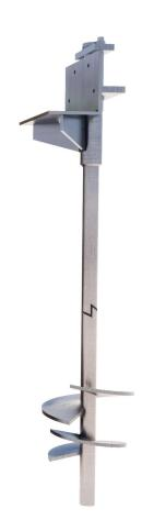
Helical piers work by transferring a load of a structure from unstable or poor soil to more stable soil or bedrock. The helically-shaped blades on the pier act as screws, providing a secure connection between the pier and the ground. The pier is then connected to the structure, allowing the load to be transferred to the pier and away from the unstable soil. This can provide a more stable foundation for the structure and can help to prevent foundation settlement and other damages.
