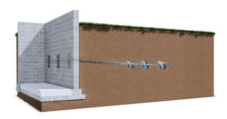
Helical tiebacks offer a solution to stabilize and straighten basement walls with significant damage from hydrostatic pressure. Installed from inside the basement, they minimize disruption to the yard and landscape. With no pressure applied during installation, hydraulic torque monitoring ensures correct installation for permanent wall stabilization. Their flexible tension adapter design allows tiebacks to securely anchor into various wall structures.
